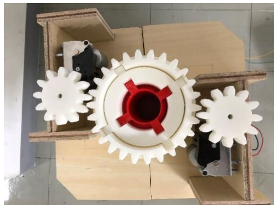
Fig.21 Placement of two motors and walls
