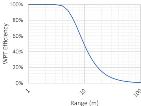
Fig. 8. WPT Range vs. Predicted Efficiency
