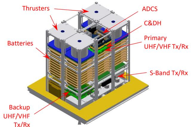
Fig. 4. Core Structure Subsystems (panels not shown)
