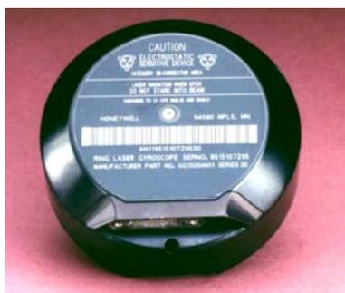
図 4-2 GG1320 AN Digital Laser Gyro
