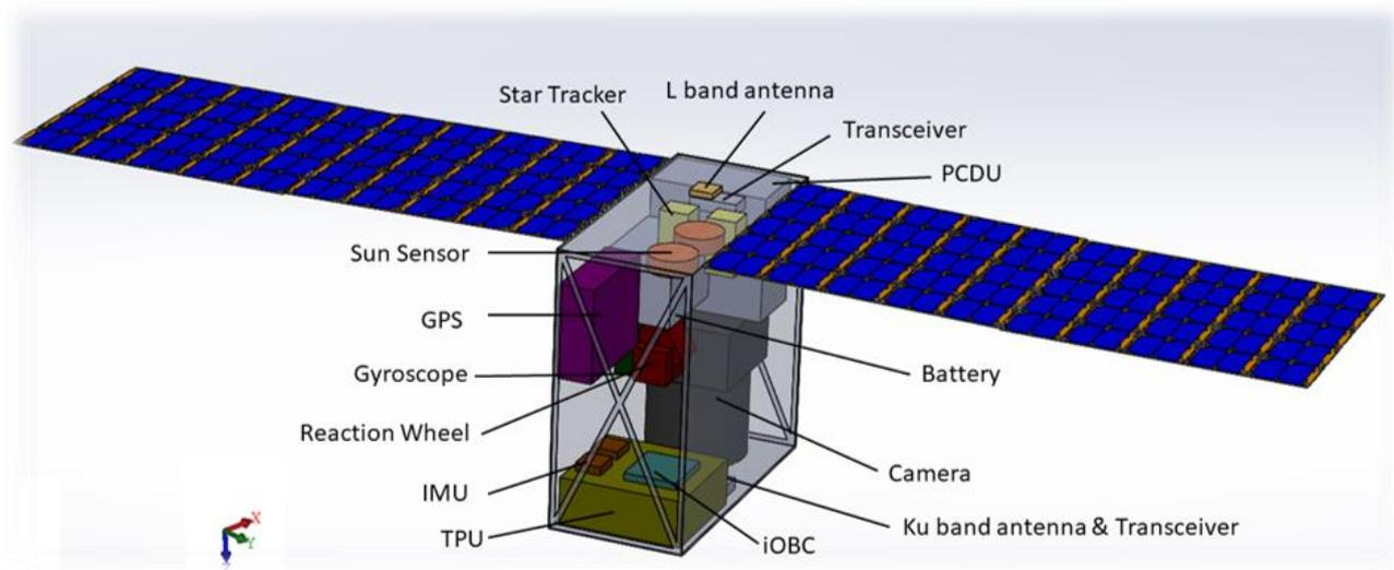
Figure 2.2 The major instruments of the ALICE microsatellite
