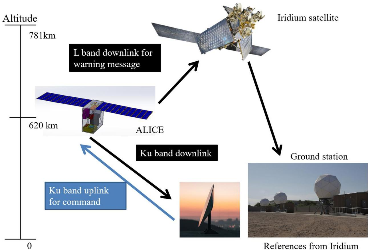
Figure 2.7 TT&C schematic diagram
