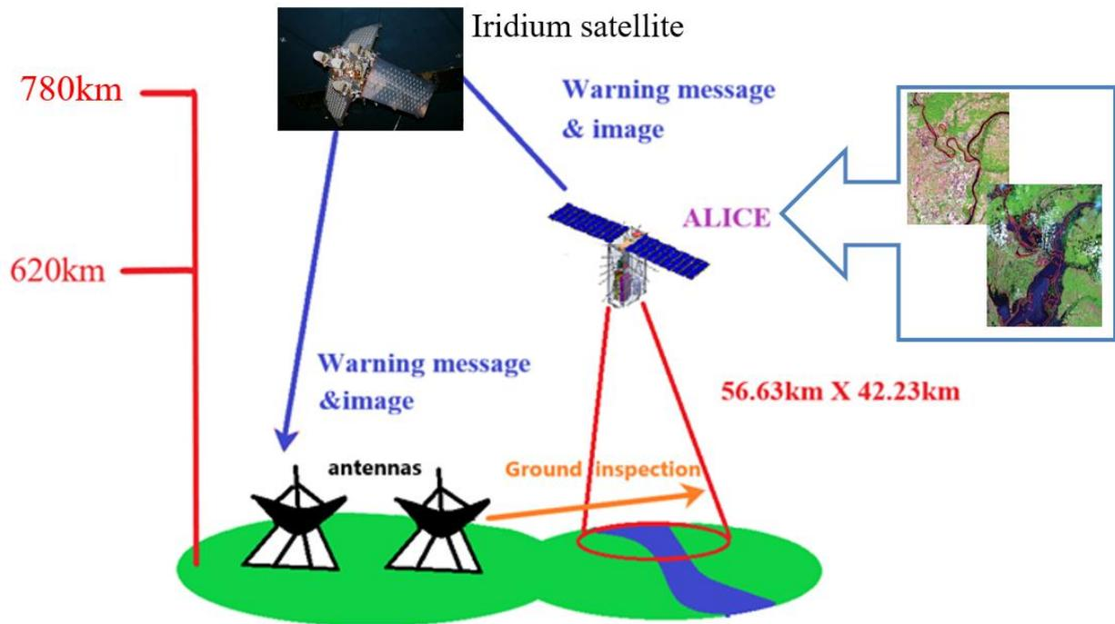
Figure 1.4 The schematic diagram of the ALICE mission
