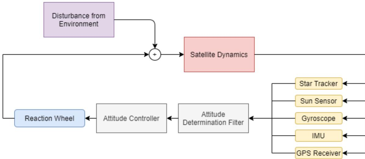
Figure 2.6 The architecture of ADCS in the ALICE satellite
