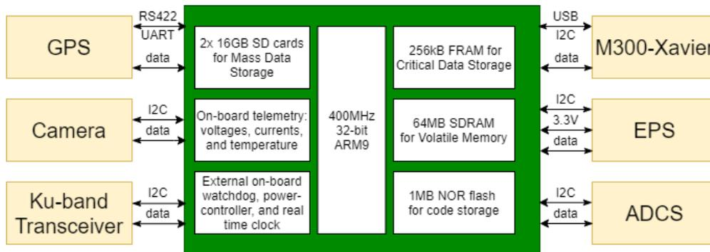
Figure 2.9 The functional block diagram of iOBC
