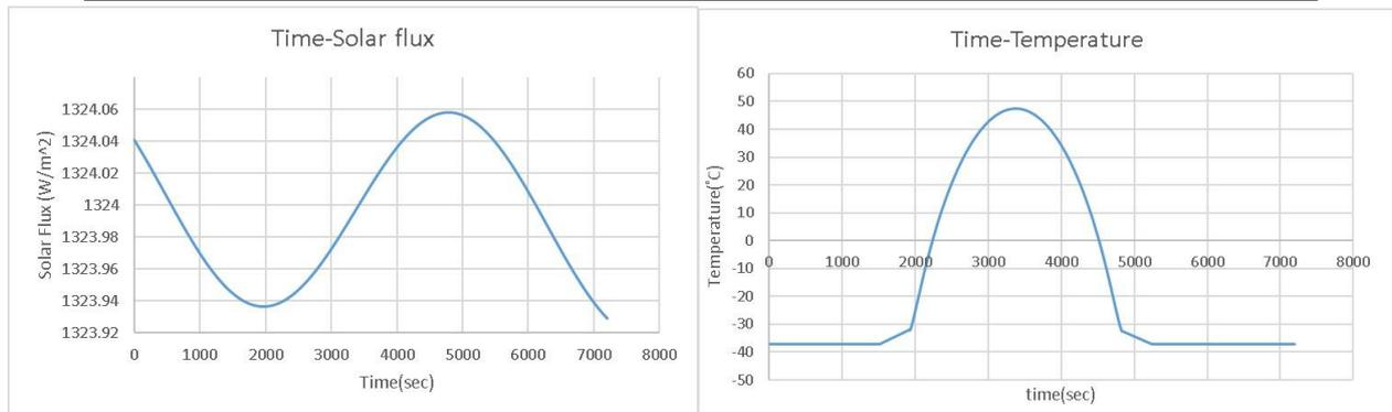
Figure 2.4 The change of Solar flux in one period (left) and the satellite temperature change in one period(~98mins) (right)
