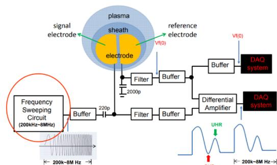
Fig 2. System configuration of TeNeP (Jiang et al., 2014)
